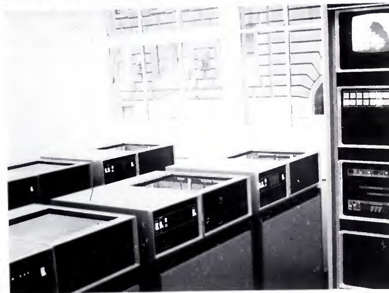
CMX-600 at EUE-Screen Gems; editing console (top), computer control and tape decks (bottom).
